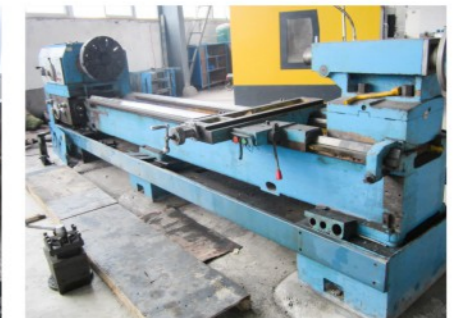
安阳6180三米改数控 Anyang 6180 three meters upgraded CNC Type
