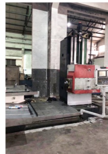
俄罗斯T130镗床改数控 Russian T130 boring machine changed to CNC type
