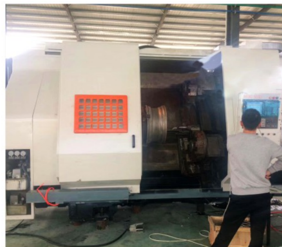
德国双通道轮毂车改造 German two-channel wheeled car transformation
