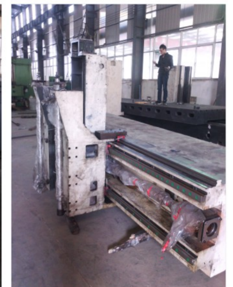
6米龙门改造 6m gantry boring and milling machine upgraded CNC Type
