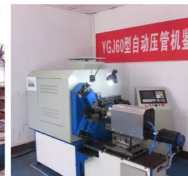
中建二局用压管机改造 China construction Crimping Machine renovation
