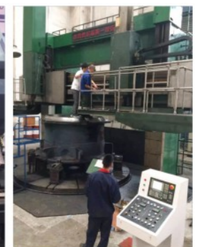
齐齐哈尔第一机床厂五米立车改造 Qiqihar five meter vertical lathe upgraded
