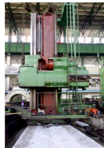
斯柯达200十米落地镗改数控 Skoda 200 ten-meter floor boring machine changed to CNC type
