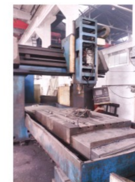
2218龙门改造 2218 Gantry boring and milling machine upgrade
